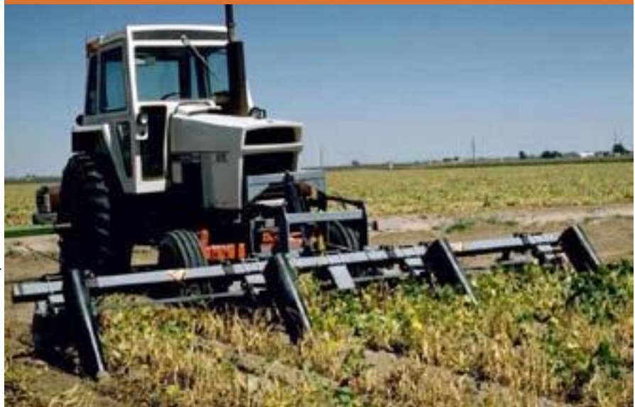
Figure 14-2. Tractor-driven cutter used to harvest dry beans.
